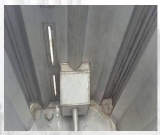
These Tanks were specifically designed & built to Chevron Standards for toughness & durability, inside we have filter fitted to the outlet & baffle to avoid too much movement of the interior liquid. Outlet tap is sunk into the tank to avoid unwanted collisions with other equipment. Triple site glass to always maintain visual levels. These tanks come with complete MDR's, slings & shackles & load test certification.
